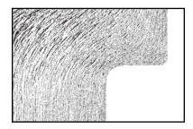
Controlled head forging, uniform grain flow, unbroken flow lines; makes heads stronger; minimizes failure in vital fillet area; adds to fatigue strength.
