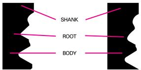
CONVENTIONAL THREAD RUNOUT – Note sharp angle at root where high stress concentration soon develops crack which penetrates into body of the screw. UNBRAKO "3-R" (RADIUSED ROOT RUNOUT) THREAD -
